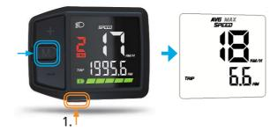
The screen will switch to the 'data clear' mode, alternately showing Max/average speeds and the trip meter.
