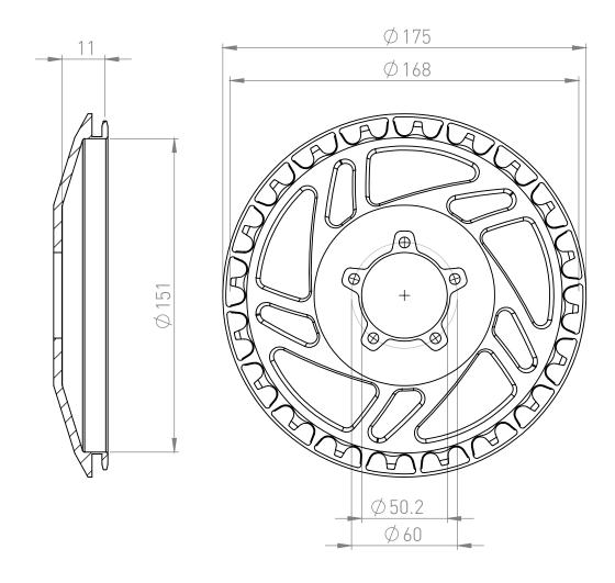
Note the package includes a 2mm Spacer so that you can space the Bling Ring out to the same offset as the original Bling Ring offset. We decided to offset the Bling Ring an extra 2mm so that users could try get that perfect chainline for the 73mm BB frames. If you are building a 73mm BB frame try installing without the spacer. You should have at least 1.5mm gap between the ring and chain-stay.
