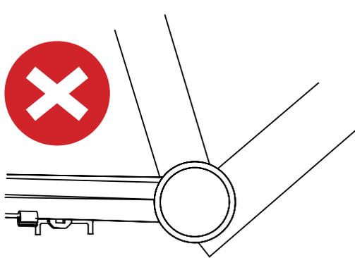
Protruding tubes, Chain guide mounts or welds may get in the way of the motor.
