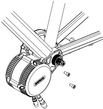
5. Unscrew to the motor from the Motor Plate and slide the motor out.
