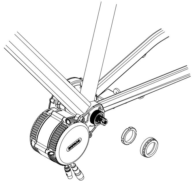
8. Install the stock Bafang lock rings and carry on with your build like a normal conversion.
