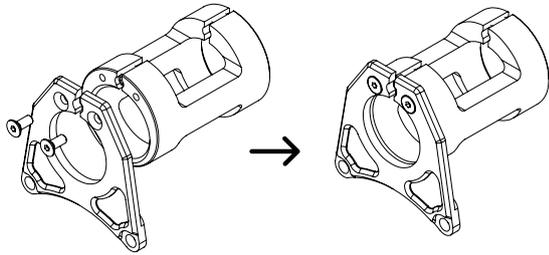
**1. Assemble the Motor Plate to the Adapter. Use a drop of Loctite onto the Motor Plate Screws then tighten to 3Nm.**
