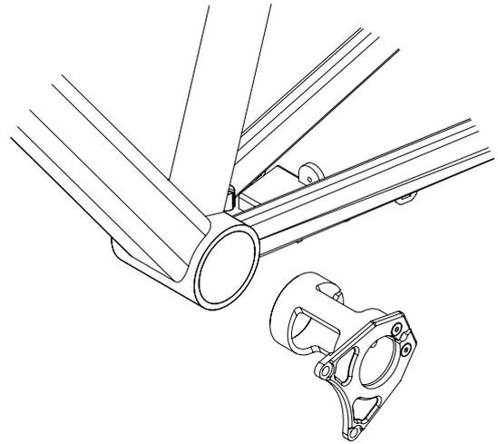
**2. Slide into frame from the left side and push hard against the frame. It should be rotatable.**
