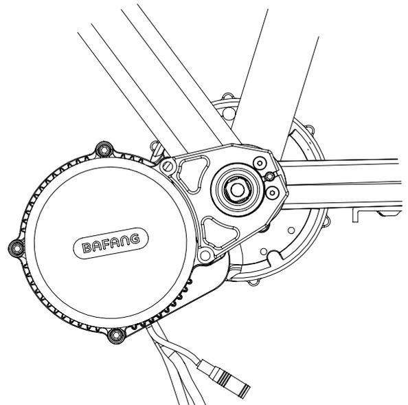
**4. Rotate the motor up until it stops on the frame, hold and tighten the left Exapander Screw. This will expand the adapter.**
