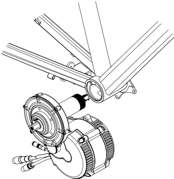
**3. Slide your motor in from the right side. install the M6 bolts you would usually use for the stock plate and screw the motor to the Motor Plate.**
