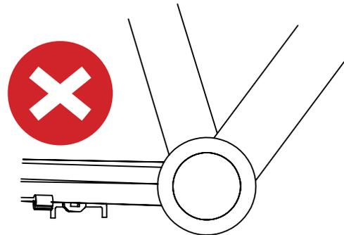
Carbon frames often have a lot of reinforcing under the BB of the frame the motor can not fit
