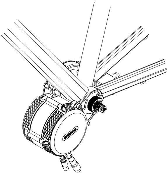
7. Slide your motor in from the right side and attach the motor back on to the Motor Plate using the M6 screws. Tighten to 9Nm.
